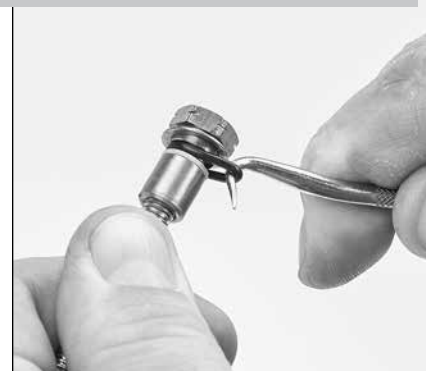
1.21 Using a pick, remove the plunger retainer O-ring from plunger retainer.
