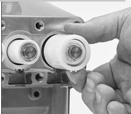
1.39 Install seal retainer with tabs facing down.
