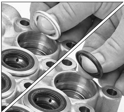
1.41 One side of the V-packing has a groove. Install the first V-packing with the groove side facing down and press into place.
