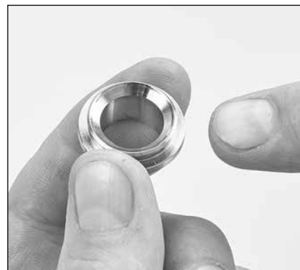
2.10 Inspect tapered surface of valve seat for wear, pitting or damage.
