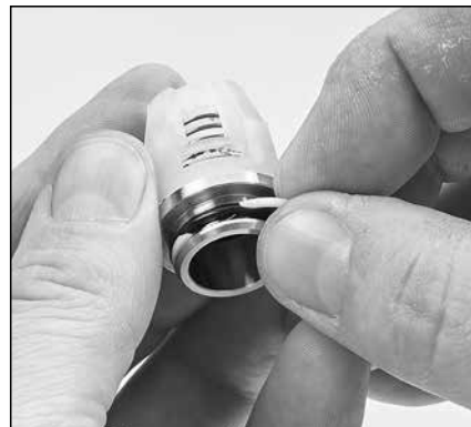
2.18 Replace valve seat O-ring into the top of the groove, then backup ring at the bottom.
