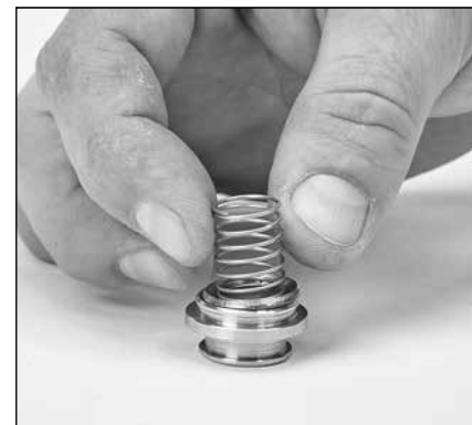
2.15 Place spring onto concave side of valve.
