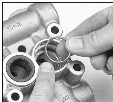
1.14 Remove the male adapter and inspect for wear or damage.
