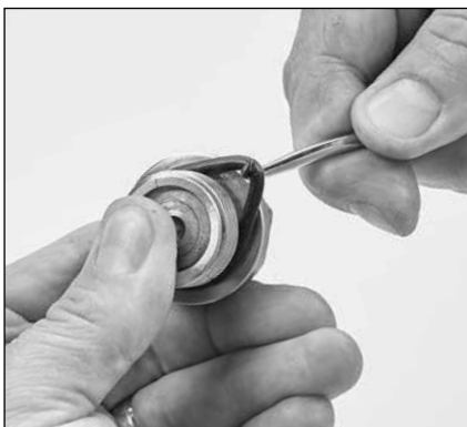
2.02 Using a pick, remove O-ring from valve plug.
