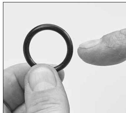
2.03 Inspect valve plug O-ring for cuts, nicks or damage.
