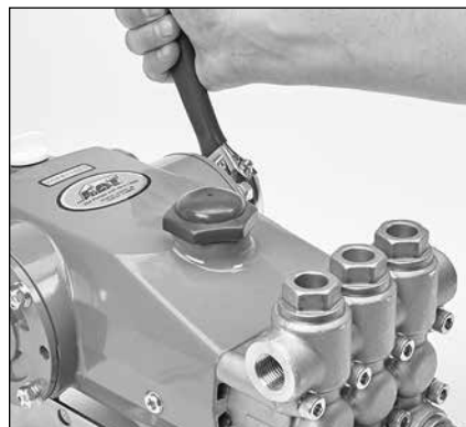
1.51 Rotate crankshaft with adjustable wrench to ensure proper movement of plunger rod assemblies and that seals are not binding.
