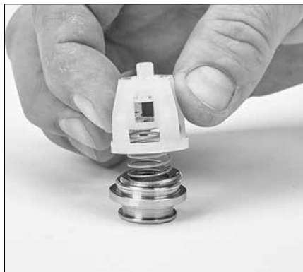
2.16 Place spring retainer onto valve seat.
