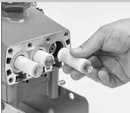
1.19 Remove the plunger and retainer.
