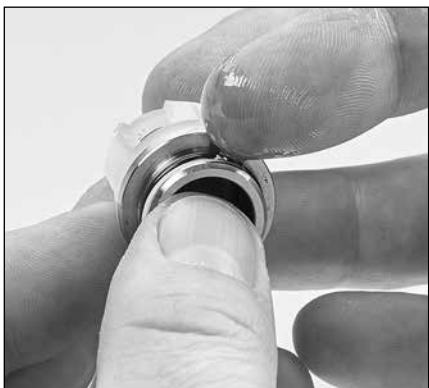
2.19 Apply a lubricant to outside surface of the valve seat O-ring.
