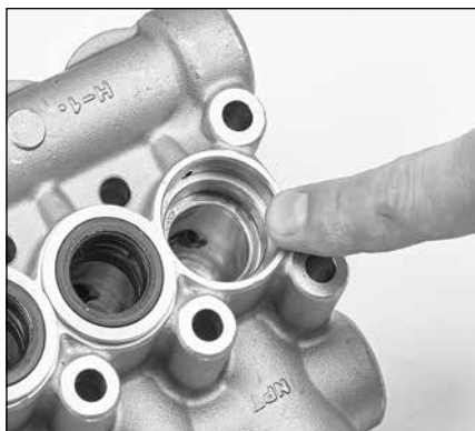
1.15 Inspect the manifold bore to ensure sealing surface is smooth and free from corrosion.
