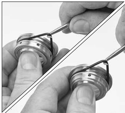
1.09 Using a pick, remove the seal case O-ring.
