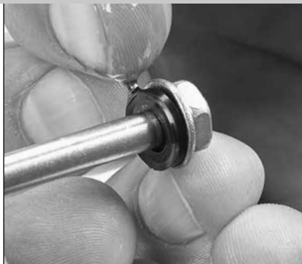
1.34 Apply a lubricant to outside surface of the seal washer.
