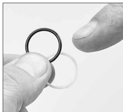
2.12 Inspect valve seat O-ring and backup ring for cuts, nicks, or damage.
