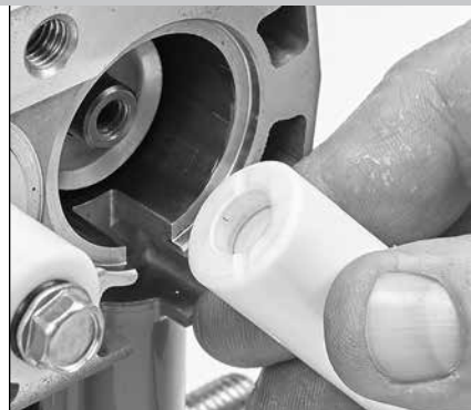
1.35 Look for stepped side of plunger. This side goes towards the pump crankcase.
