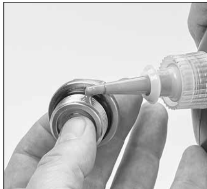
2.22 Place a drop of Loctite® 242® on the threads of valve plug.
