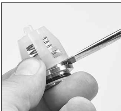
2.06 Place flat tip screwdriver in gap and twist to completely separate.
