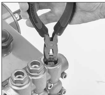
2.04 Use a needle-nosed pliers to grasp the top of the spring retainer. Twist while pulling away from manifold to remove valve assembly.
