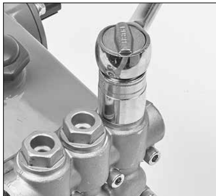
2.24 Using a 27 mm hex socket with ratchet, tighten valve plugs. Torque to 870 in-lbs, 72.5 ft-lbs, or 98 Nm.
