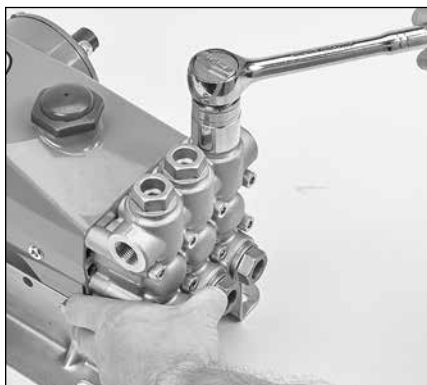
2.01 Use a 27 mm socket with ratchet to remove the valve plug from pump manifold.
