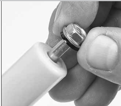
1.36 Insert plunger retainer with seal washer into non-stepped side of plunger.
