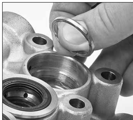
1.40 Install the male adapter with the flat side facing down.
