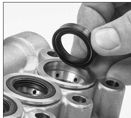
1.45 One side of the low-pressure seal has a groove and spring. Install groove side facing down and press into place.
